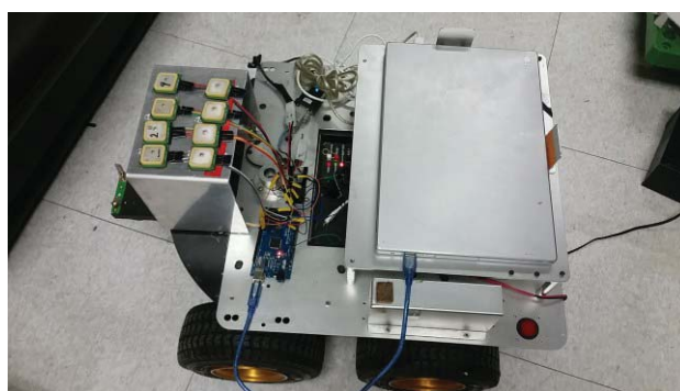
Fig. 1. Sensor system attached to a mobile robot
